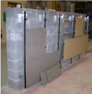
Ventilated rainscreen mockups in IMI's Addison training center helped lead to the use of this system on the interior and exterior walls on the First Bank and Trust in Skokie, Illinois, installed by Trowel of Excellence™ certified contractor DTI of Illinois.
